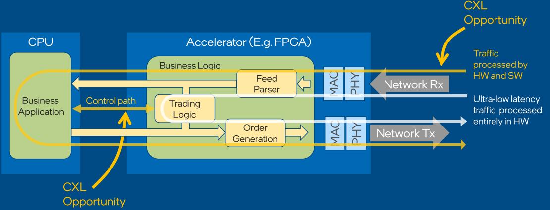
CXL enables tightly coupled CPU-HW interactions, resulting in better use of CPU and hence helping reduce accelerator complexity
