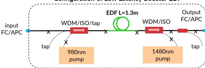
**Acronyms:** NF is noise figure; m is meter; nm is nanometer; L is length; WDM is wavelength division multiplexing; EDF is erbium doped fiber; ISO is isolator
