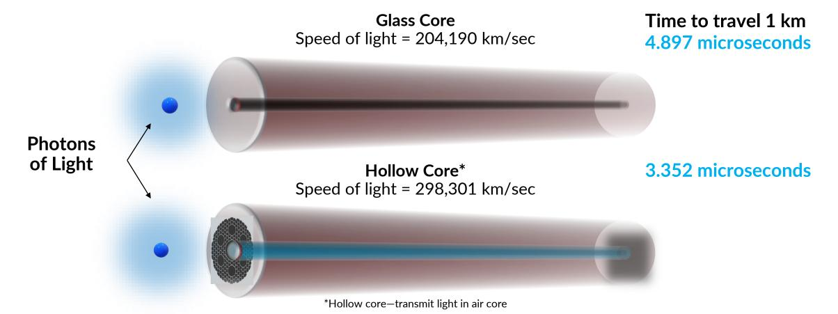
The Challenge: to realize the latency improvement in field deployed networks because the fiber (i.e., hollow core) is intrinsically sensitive to external stress.
