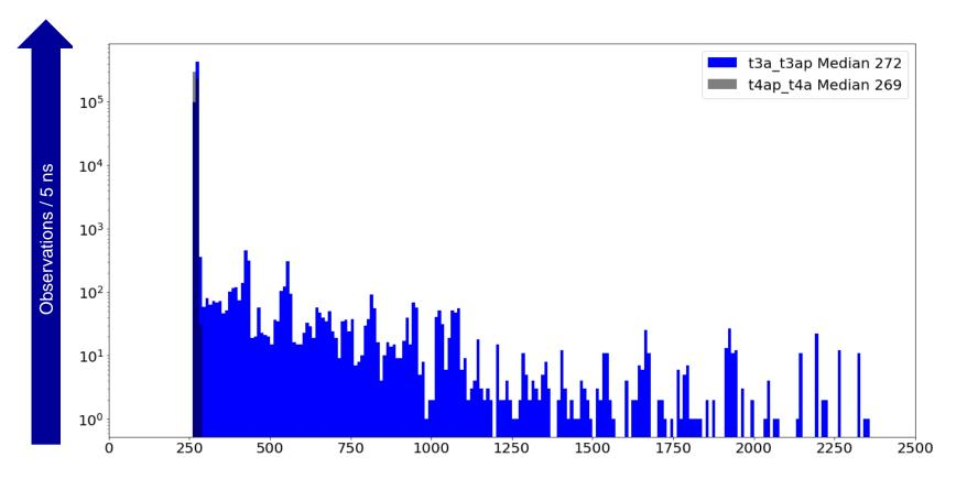
Nanobursts lead to queuing depending on number of packets and packet size.
