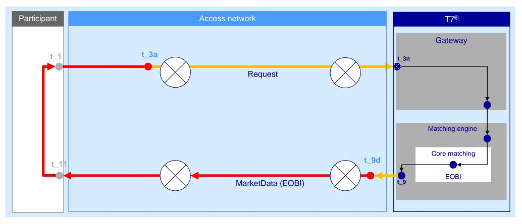
FESX => FDAX Reaction time based on T7<sup>®</sup> times (t\_9 to t\_3n)\*
